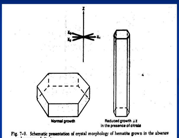
Fig. 7-9. Schematic presentation of crystal morphology of hematite grown in the absence and presence of citrate.
